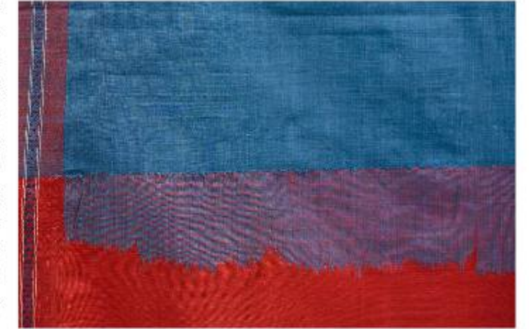
Interlocking Kondi technique for pallu and body
